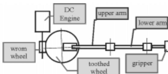
Fig. 3. The corresponding abstract design with skeletal, engine and hinge elements to the grab arm.
