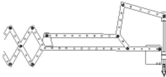
Fig. 4. Hunveyor-2 soil hardness measuring arm. Left: the end of the telescopic segment, at right end is the drill.
