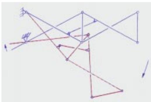
Fig. 1. Unusual connection of console elements results in nonlinear motion at the end of the console.
