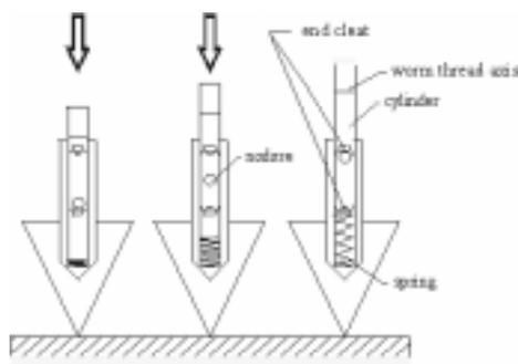
Fig. 5. The 3 stages of the drill at different soil hardness. Left: hardest soil, center: middle soil hardness, right: loose soil.
