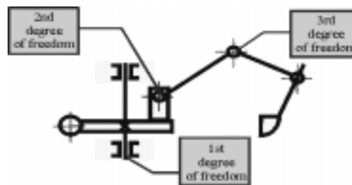
Fig. 2. The structure of a grab arm with 3 degrees of freedom and with extended maneuvering space.
