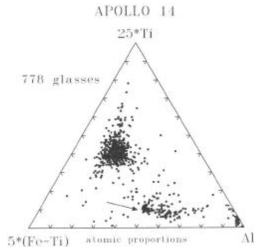
**Figure 2.** Glass compositions (778) from regolith 14259 and 5 regolith breccias (14047, 14049, 14301, 14307, 14313). The highland basalt glasses are identified with an arrow.
