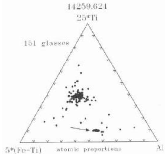
**Figure 1.** Glass compositions (151) from regolith 14259. The highland basalt glasses are identified with an arrow. The coordinates of the ternary diagram represent the atomic proportions of the non-volatile elements analyzed in the lunar impact glasses and can be used to describe the chemical and mineralogical nature of the original target materials [3].
