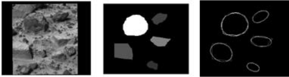
Figure 1 a) Original image taken from the Mars Pathfinder landing site, b) rocks identified from image, c) ellipses fitted to rock outlines.
