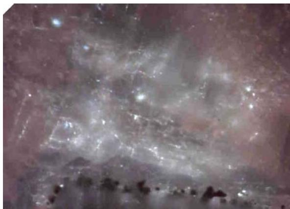
Fig. 2. Hydrocarbon inclusions fluorescing under U-V light in vein calcite. Each inclusion 5-10 microns size.
