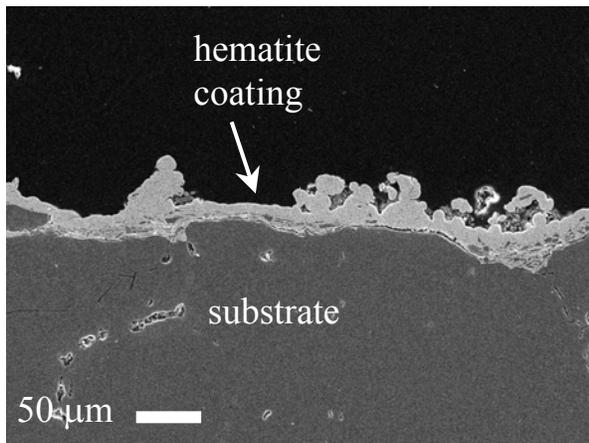
**Figure 3: Hematite coating.** SEM cross-section image of a hematite film that formed on a quartz substrate. SEM images measured of different areas of the sample show that the coating is  $\sim 10\text{--}40\ \mu\text{m}$  thick. This sample (bhm3) was from near Bunker Hill Mine, eastern Inyo Mountains, Saline Valley, Inyo County, California.
