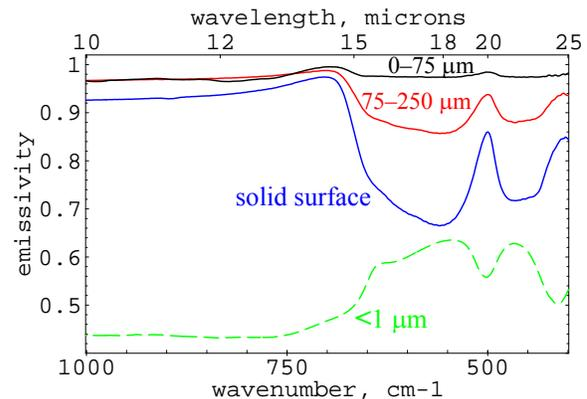
**Fig. 1. Surface vs. volume scattering.** Surface scattering dominates the “solid surface” spectrum, causing reststrahlen emissivity troughs. Volume scattering dominates the optically thin,  $<1\ \mu\text{m}$  particles, causing emissivity peaks. Volume scattering contributes to the spectral contrast decrease in the 75–250  $\mu\text{m}$  and 0–75  $\mu\text{m}$  samples. Sample “hematite.1”, from [6], shown in 1 - biconical reflectance (upper traces) or 1- transmission (lower trace).
