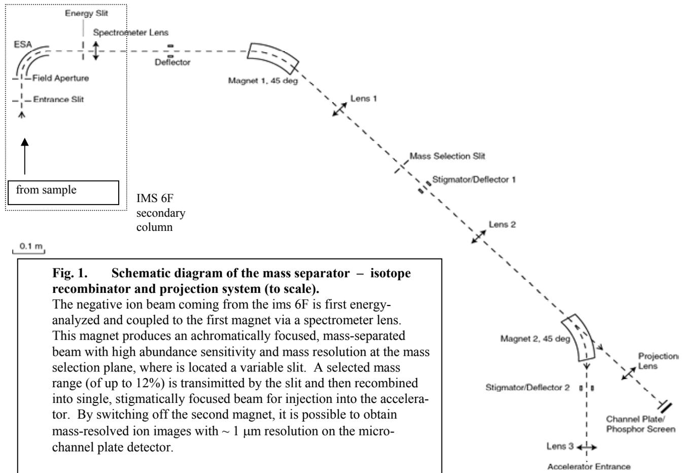
**Fig. 1. Schematic diagram of the mass separator – isotope recombinator and projection system (to scale).**
