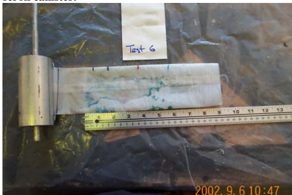
Figure 3 Injected particles deposited along the filter in sequence.
