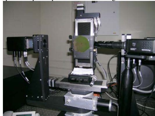
Figure 5: Variable Angle Spectroscopic Ellipsometer with full hexagon wafer mounted for analysis.
