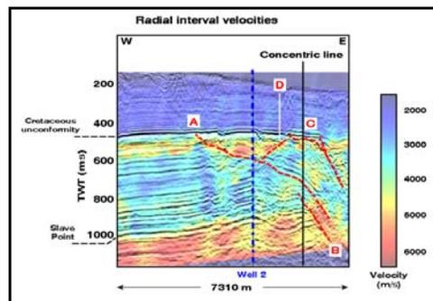
Figure 4. Overlay of radial line interval velocities on post-stack time migration.
