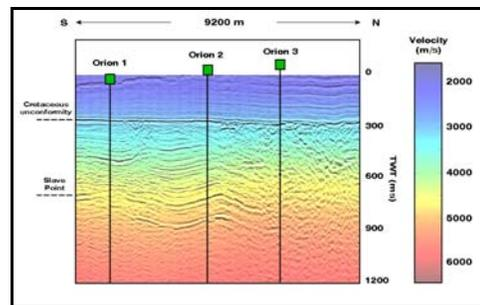
Figure 2. Overlay of a 2D section from the 3D tomographic model for the concentric line on post-stack time migration.
