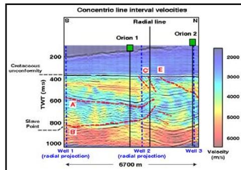
Figure 3. Overlay of concentric line interval velocities on post-stack time migration.
