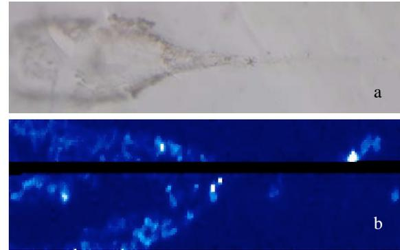
Figure 1. (a) Optical micrograph showing a carrot-shaped track from a hypervelocity impact of a chondritic particle in aerogel deployed on the Russian Space Station *Mir*; (b) An Fe fluorescence map ( $470 \times 140 \text{ }\mu\text{m}$  at  $2 \text{ }\mu\text{m}$  pixel resolution) showing Fe-rich material deposited in the track, as well as a terminal particle (ALS X-ray Micro-diffraction Beamline). Black stripe pixels are missing data.
