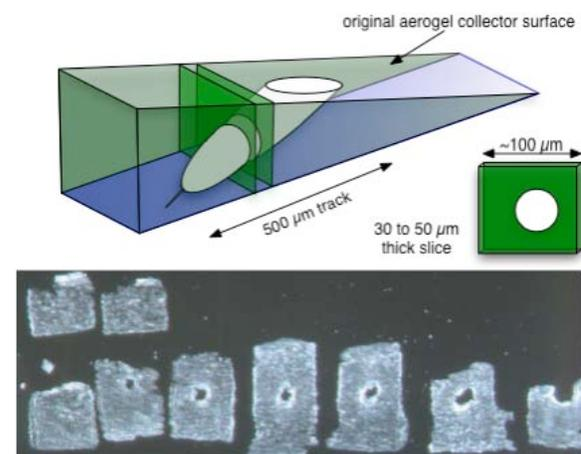
Figure 2. Schematic representation of an aerogel "keystone" extraction of an entire event from the aerogel collector. The track has been sliced across to produce 9 wafers  $<50\text{-}\mu\text{m}$  thicknesses
