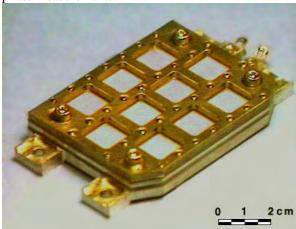
The API-S sensor carries out both send and receive operation through a single transducer array. The transducer array is driven by a 10ms long pulse of 20V peak to peak 1MHz square waves, resulting in a transmitted
