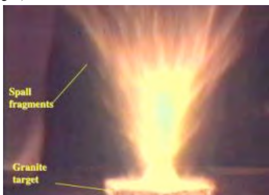
Fig. 2. High-speed video frame of impact.
