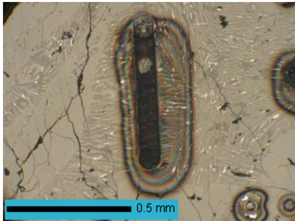
Fig. 4 Image showing the area of raster analysis of the quenched matrix of 15499.
