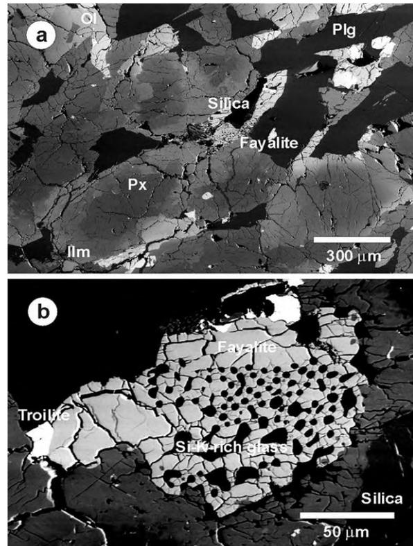
Figure 3. (a) BSE image of the texture of basaltic Clast A olivine (Ol), extremely zoned pyroxene (Px), plagioclase (Plg), ilmenite (Ilm), silica (Silica) and fayalite (Fayalite). (b) BSE image of fayalite contains inclusions of Si-K-rich glass.
