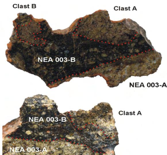
Figure 1. Photograph of two sections of specimen Northeast Africa 003-B lunar basaltic breccia.
