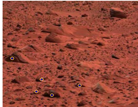
Figure 1. Candidate instrument targets automatically selected in MER Pancam Image from Legacy site. All five of the automatically selected targets are rocks. The expected number of blindly selected rock target points is less than one of five. Only points within 9m of the rover were considered as this is the range of the ChemCam instrument.
