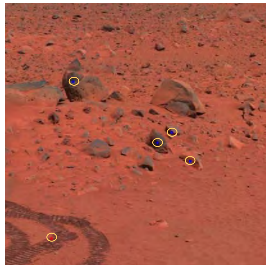
Figure 2. Candidate instrument targets automatically selected in Legacy Pancam image with one miss. Four are correctly rocks, while one is a site in the disturbed soil of the rover track. Note that the selecting the largest rocks was not a criterion.
