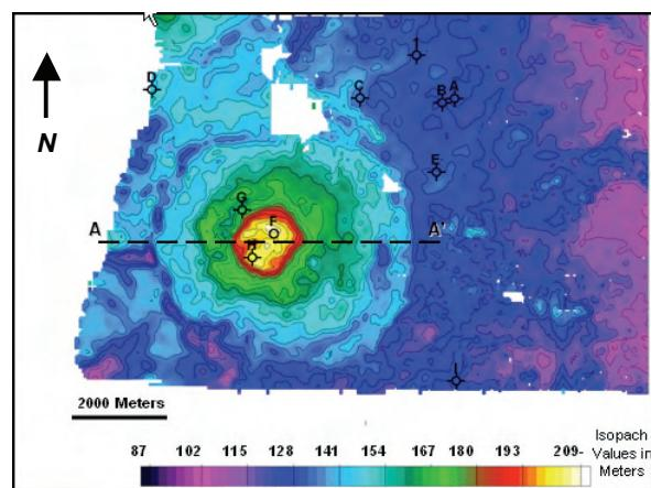
**Figure 1.** Isopach map of potential crater infill, between upper Nortonville Shale marker (blue line, Fig. 3) and base Nortonville Shale/top Domengine Formation marker (red line, Fig. 3). Colored isopach scale is in meters. West-to-east seismic profile line A-A’ (Fig. 3) is indicated; other letters correspond to well locations.
