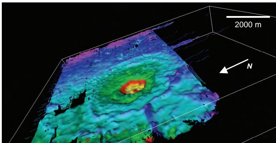
**Figure 4.** Oblique, inverted 3-D-view isopach map of potential crater infill. Map is based on same isopach interval as in Figure 1, between upper Nortonville Shale and base Nortonville Shale/top Domengine Formation markers. Vertical exaggeration is 20X. Isopach colors and thicknesses are the same as in Figure 1. Note north arrow.
