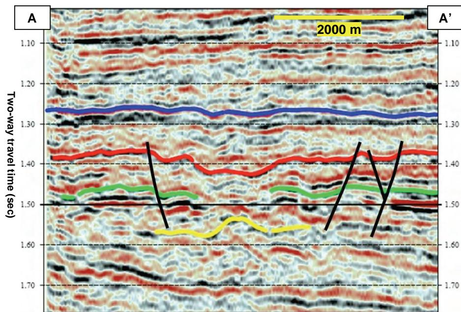
**Figure 3.** West-east seismic profile across structure (A–A', Figs. 1–2). Stratigraphic markers: Blue—upper Nortonville Shale; red—base of Nortonville Shale/top of Domengine Formation; green—lower Domengine Formation; yellow—approximate base of Capay Formation/top of Mokelumne River Formation. Selected major, concentric normal faults (Fig. 2) that intersect the profile are shown schematically by black lines.
