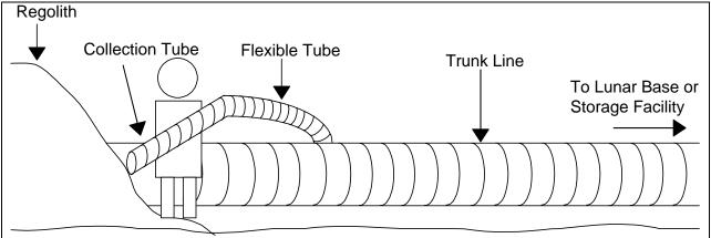
**Figure 2**. Conceptual drawing of possible method of collecting lunar soil using the "Lunar Soil Magnetic Collector" (LSMAC). The astronaut/robot uses a slightly flexible coil 'sucker tube' to collect soil, which is in turn fed into a "Trunk Line" that is capable of higher flow rates, these trunk lines are also movable. Multiple collection branches would feed into one trunk line.
