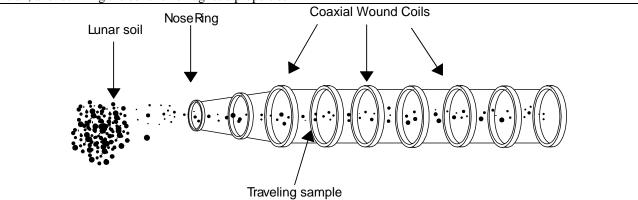
**Figure 1**. Diagram of our "Lunar Soil Magnetic Collector". Coaxial rings are sequentially powered up and down in a rippling effect to move ferromagnetic lunar soil to the right.
