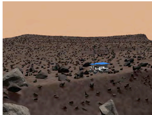
Figure 2. A test director's view of the simulated prototype rover in a SimScape terrain viewed in ROAMS.
