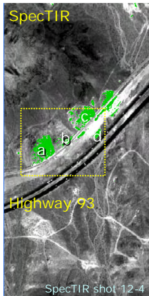
Fig. 5: Mapping of an alunite signature (green) in SpecTIR hyperspectral imagery. Gray image shows the 0.554 \mu\text{m} channel. Both SEBASS and SpecTIR map signatures in this region that match alunite. The dotted box marks the location shown in Fig. 6. Signature mapped is from the USGS Speclab library, “alunite1” (Fig.3). The Fig. 1 picture is at location “c” in this figure.
