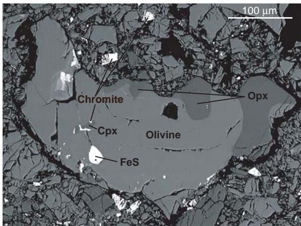
Figure 1: Backscattered electron image of olivine-diogenite MIL03443. Major phases are (in order of abundance in the thin section) olivine (light grey), chrome-spinel (white), and orthopyroxene (dark grey). The bright spots within the olivine and opx are sulfide inclusions. Notice the undulating boundary between the olivine and opx.
