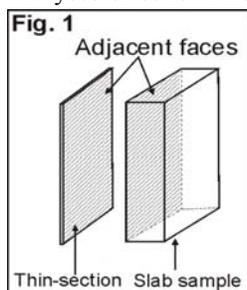
Lunar mare basalts, chosen for their representative nature to an Apollo landing site, were cut such that a thin-section could be prepared directly opposite the bulk portion of the rock (Fig. 1). The opposing rock slab was used for preparation of clean mineral separates. This arrangement of thin-section and chip was used to aid in the correspondence of the mineralogies. The chemistry of the minerals was fully characterized in both the thin-sections and the mineral separates.
