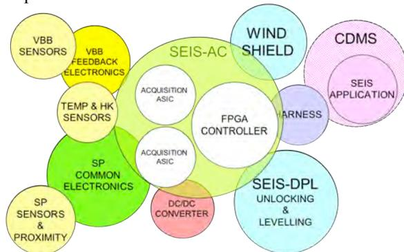
Fig 2. Instrument schematics
