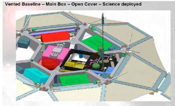
Fig 1. Example of SEIS accommodation (courtesy Thales-Alenia-Space). The SEIS is the red cylinder located near the center of the lander platform
