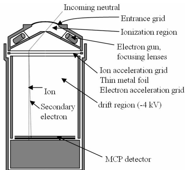
**Figure 1.** Mass spectrometer design.
