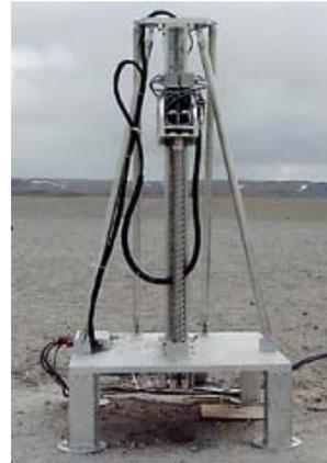
Figure 5. The DAME drill was deployed three times in the Arctic field tests (2004, 2005 and in 2006) on Devon. The drill uses 1.75 inch full faced bit for cutting material and auger for cuttings removal.
