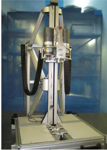
Figure 3. Honeybee CRUX drill was designed for three different drilling modes: rotary, rotary-percussive and percussive. The augers and drill bits are not shown.
