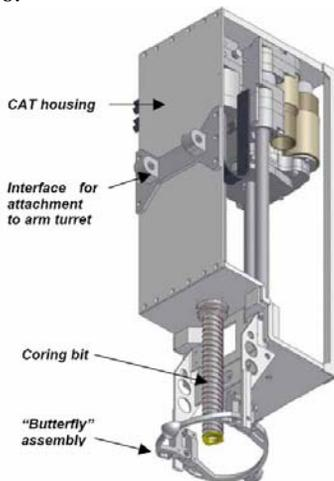
Figure 1. Components of the Corer-Abrader Tool in coring mode.
