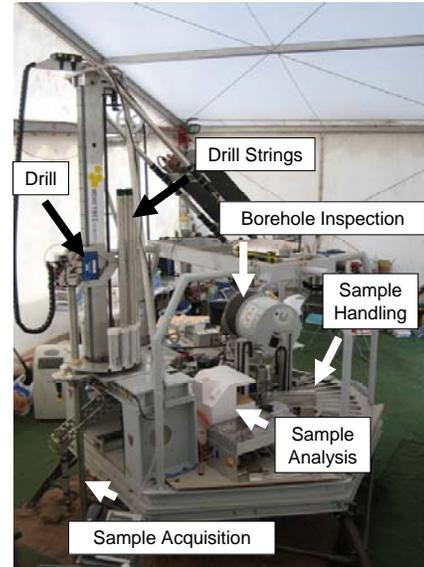
Figure 4. The MARTE (Mars Astrobiology Research and Technology Experiment) science package with all the instruments and a drill.
