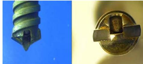
Figure 2: Detail of Sampling Tip (Door Closed) of the Sample Acquisition and Transfer Mechanism (SATM) drill.
