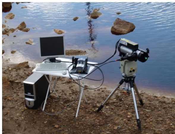
Figure 2. Picture of the remote Raman instrument. Background Rio Tinto, Spain. Credit T. Acosta
