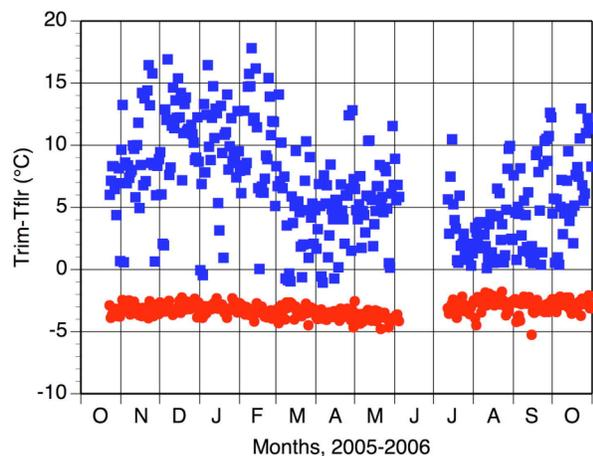
Figure 1. Daily maximum (blue) and minimum (red) temperature differences between the rim and floor of Meteor Crater from 22 Oct 2005 through 31 Oct 2006. Note missing data between 4 June and 11 July.
