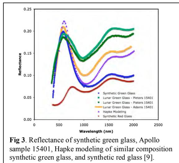
**Fig 3.** Reflectance of synthetic green glass, Apollo sample 15401, Hapke modeling of similar composition synthetic green glass, and synthetic red glass [9].
