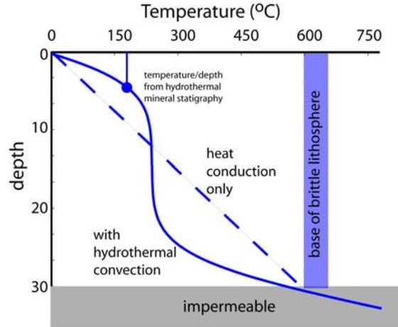
Figure 3. Hypothetical crustal thermal structure with hydrothermal cooling consists of relatively uniform temperature where heat is transferred convectively between conductive thermal boundary layer at the top and bottom. In this case the surface thermal gradient is about twice the purely convective gradient (dashed line) corresponding to  $Nu \sim 3$ .
