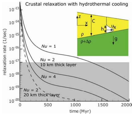
Figure 2. Effect of hydrothermal cooling on the relaxation rate of crustal thickness variations due to thermally-activated creep near the base of a wet-diabase crust. Hydrothermally-cooled layer thicknesses of 10 and 20 km are assumed for solid and dashed curves, respectively. Relaxation rates must be less than about  $10^{-17}$ /sec (within the shaded region) to preserve crustal thickness variations to the present day, thus requiring hydrothermal cooling.
