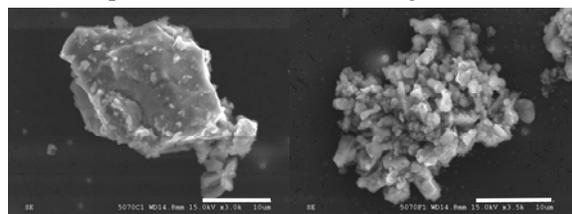
**Figure 1:** Secondary electron images of external surfaces of a compact grain (left) and a fluffy grain (right) in L1. Scale bars are  $10 \mu\text{m}$ .
