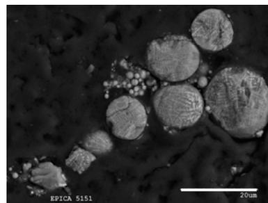
**Figure 2:** Backscattered electron image of polished sections of cosmic spherules from sample L2. Scale bar is  $20 \mu\text{m}$ .
