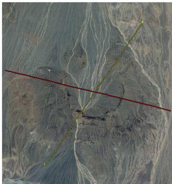
Fig. 1. Satellite image over the Tsenkher structure with the measured profiles indicated. Each profile is approximately 12 km long. They cross at the center of the studied crater structure which apparent rim is visible as a ring of hills with sharp, dark shadows at a radial distance of about 1.8 km. Profile-1 is yellow (SW-NE), and Profile-2 is red (WNW-ESE). North is up.
