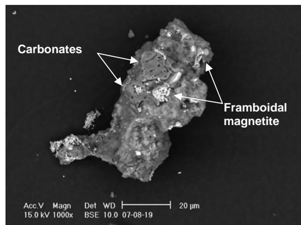
**Figure 2.** Backscattered electron image of a fragment of CONCORDIA micrometeorite #07-08-19 exhibiting carbonates and framboidal magnetite.
