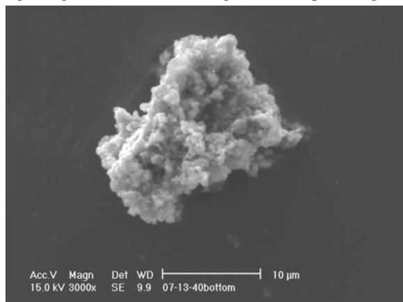
**Figure 1:** Secondary electron micrograph of a fragment of fine-grained fluffy (FgF) Concordia micrometeorite #07-13-40.
