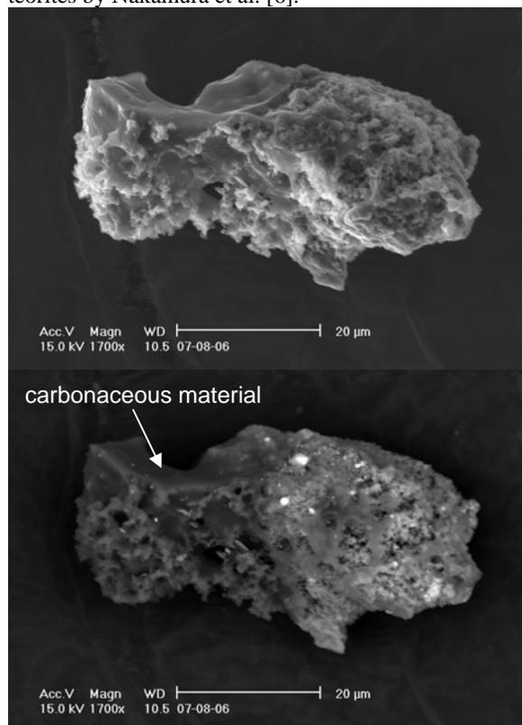
**Figure 3.** Secondary (top) and backscattered (bottom) electron images of a fragment of a fine-grained compact CONCORDIA AMM exhibiting a large amount of carbonaceous material.
