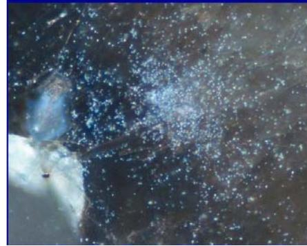
Fig. 4: A dense cluster of MTB (whitish) on brown olivine indicating an area with high concentration of submicron ferro(i) magnetic grains is seen (S-poles) (dark field). (area ca.  $100\times 100\mu\text{m}$ ).
