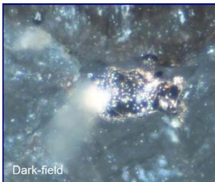
Fig. 3: Magnetic S-pole distribution on a ferrimagnetic Fe-sulphide grain (ca.  $25\mu\text{m}$ ) in Yamato 000097 as observed with MTB.
