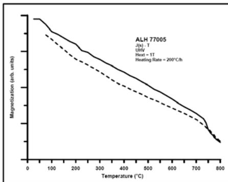
Fig. 2: Thermomagnetic curve (magnetization) obtained on ALH 77005 from 1983 with  $T_c$  of around  $760^\circ\text{C}$ , indicating Fe metal as the dominating magnetic mineral (dashed: cooling curve).
