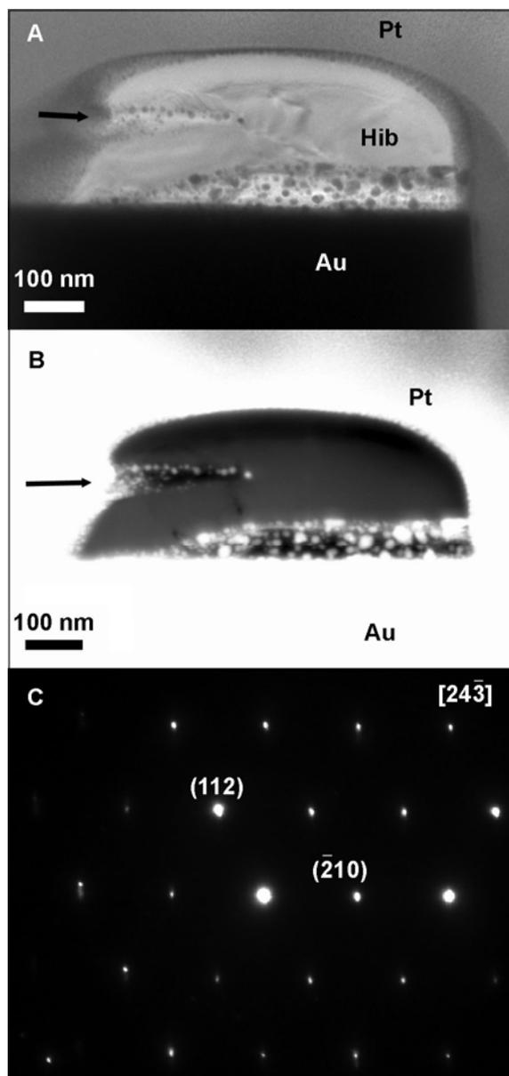
**Figure 2.** (A) Bright-field TEM image, (B) Z-contrast image and (C) selected area diffraction of supernova hibonite KH2. The arrows in (A) and (B) indicate the position of a crack in the grain. The Au nanoparticles that coat the crack and the space between the grain and Au support stub are due to redeposition of sputtered Au during the FIB processing.
