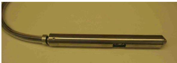
Figure 1. Measurement head unit of the new borehole instrument.
