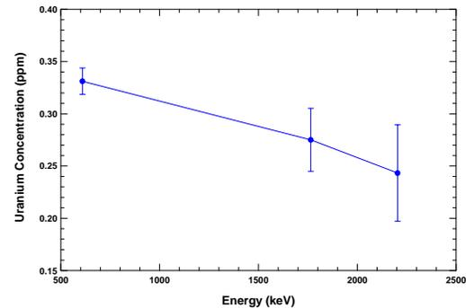
Figure 2 – Belly-band results for three Uranium peaks. The weighted mean for these peaks is 0.32 ppm.
