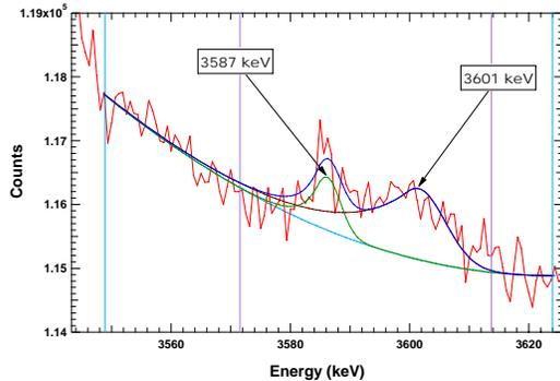
Figure 5 - Fit to the 3587 keV Sodium peak in the belly-band spectrum. The broadened peak at 3601 keV is from  $^{56}\text{Fe}(n,\gamma)$ .
