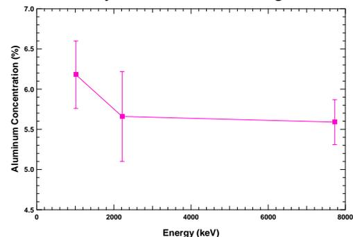
Figure 3 – Belly-band composition results for three Aluminum gamma rays. The weighted mean for these peaks is 5.8% .
