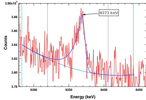
Figure 6- Fit to the 8373 keV Chromium single escape peak in the belly-band spectrum.
