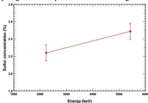
Figure 1 –Belly-band composition results for two different Sulfur gamma rays. The weighted mean of these values is 2.4% .
