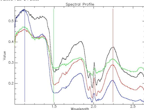
Figure 2: Representative spectra from FRT\_32F2, with simple atmosphere and  $\cos(i)$  correction. All regions, including dark layers and lower albedo upper surface units show prominent ice absorptions.
