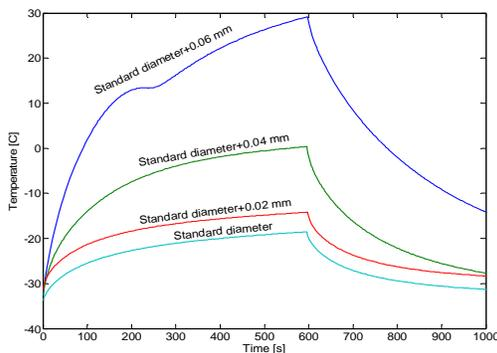
Fig.3 Time dependence of the sensor temperature for the experimental set-up shown in fig 2. Heating power  $P_H = 0.5W$ . The kink in the topmost curve results from the power system failure.
