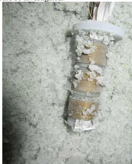
Fig. 1 The stack of thermal sensors.
