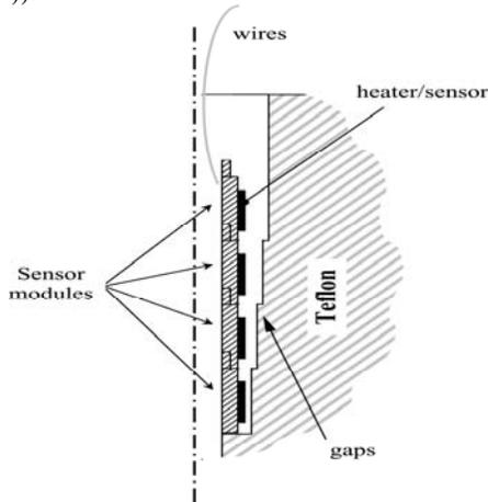
Fig.2 Sensor stack placed inside a Teflon sample.
