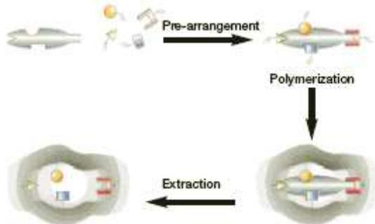
**Figure 1.** Process of molecular imprinting.
