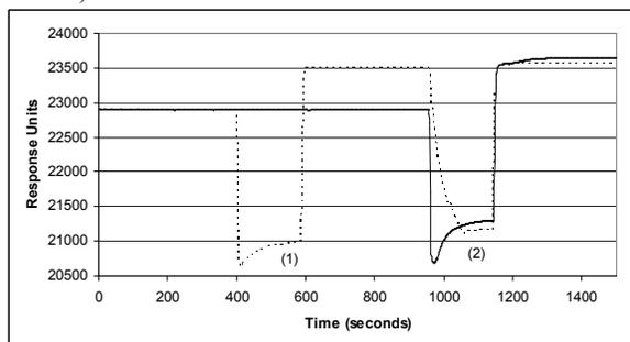
**Figure 6.** SPR sensogram detailing the competitive binding of streptavidin with a MIP. Reference channel (—); Signal channel (- -). Step 1 (400-600sec) and Step 2 (975-1175sec) display MP displacement. The reference channel was untreated with streptavidin in step 1.
