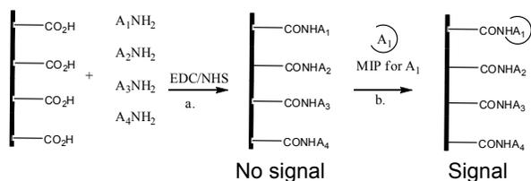
**Figure 3.** Scheme detailing the detection process.
