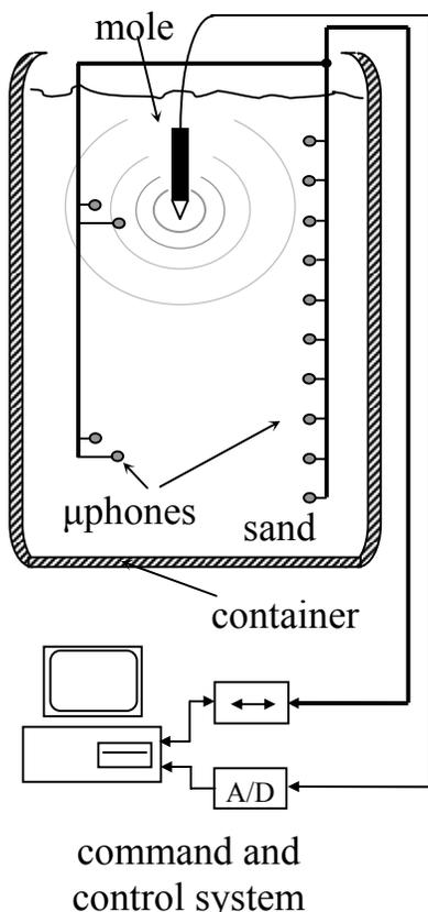
Fig. 2 Testbed system: container with dry quartz sand, passive measurements system with  $\mu$ phones, mole penetrator and the data acquisition system.
