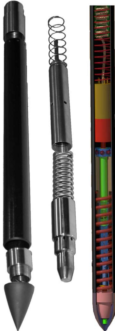
Fig. 1 The laboratory model of the mole penetrator: the outer tube with the tip (left), the hammer with the counter-mass (middle) and an artistic concept of the mole (right).
