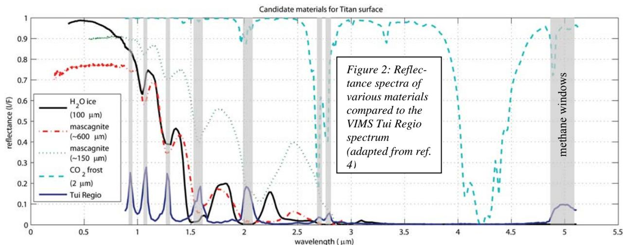
Figure 2: Reflectance spectra of various materials compared to the VIMS Tui Regio spectrum (adapted from ref. 4)
