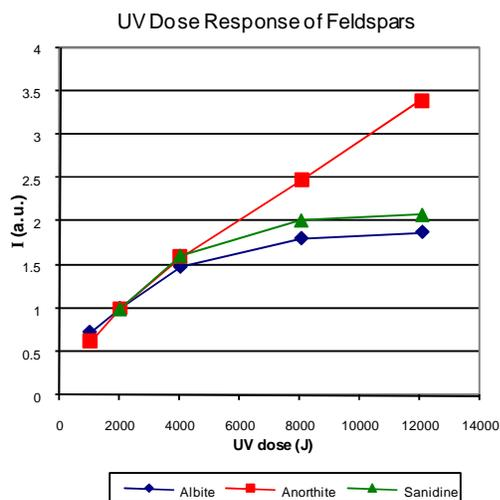
Fig. 2. OSL dose response of albite, anorthite, and sanidine feldspar samples after exposure to the deuterium source for timed increments (Exposures given in units of Joules based on lamp output in the wavelength range of 200-400 nm.) OSL measurements were conducted with blue-light stimulation and UV signal monitoring (BOSL/UV).
