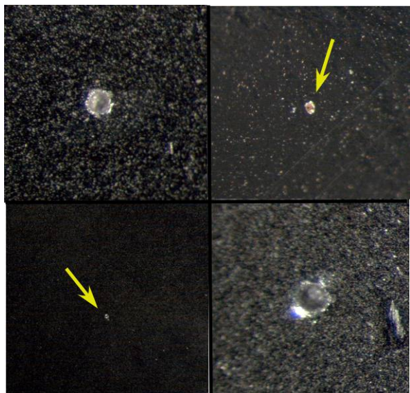
Fig. 5. Examples of microcraters on polished aluminum surface. Image on lower left has not been positively identified.
