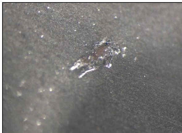
Fig. 6. Irregularly shaped gouge on aluminum kidney surface.
