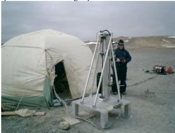
**Fig. 1. DAME planetary drill prototype at Devon Island analog test site (Haughton Crater), 2004-06.**
