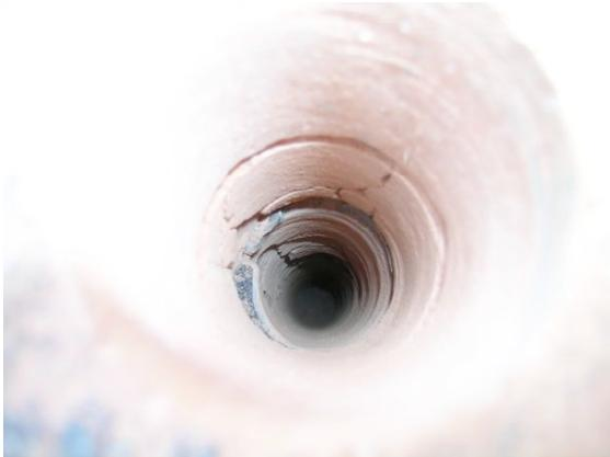
**Fig. 2. Looking downward into layers of simulant (simulated regolith, granite, basalt, bricks)**
