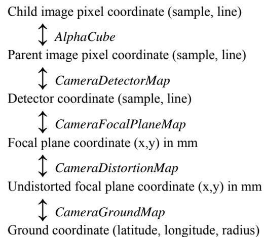
These steps are coded as five separate C++ classes: *AlphaCube*, *CameraDetectorMap*, *CameraFocalPlaneMap*, *CameraDistortionMap*, and *CameraGroundMap*, where each class computes the forward and inverse coordinate transform.
