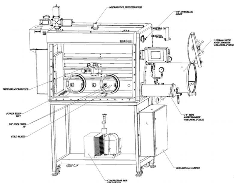
Figure 1: Glovebox design by MBraun, Inc. System includes  $-35^{\circ}\text{C}$  freezer,  $-35^{\circ}\text{C}$  cold plate, microscope, electrical connections, penetrations for gaseous nitrogen supply and exhaust, spare penetrations for future utilities and monitoring system to display and record nitrogen and temperature parameters.
