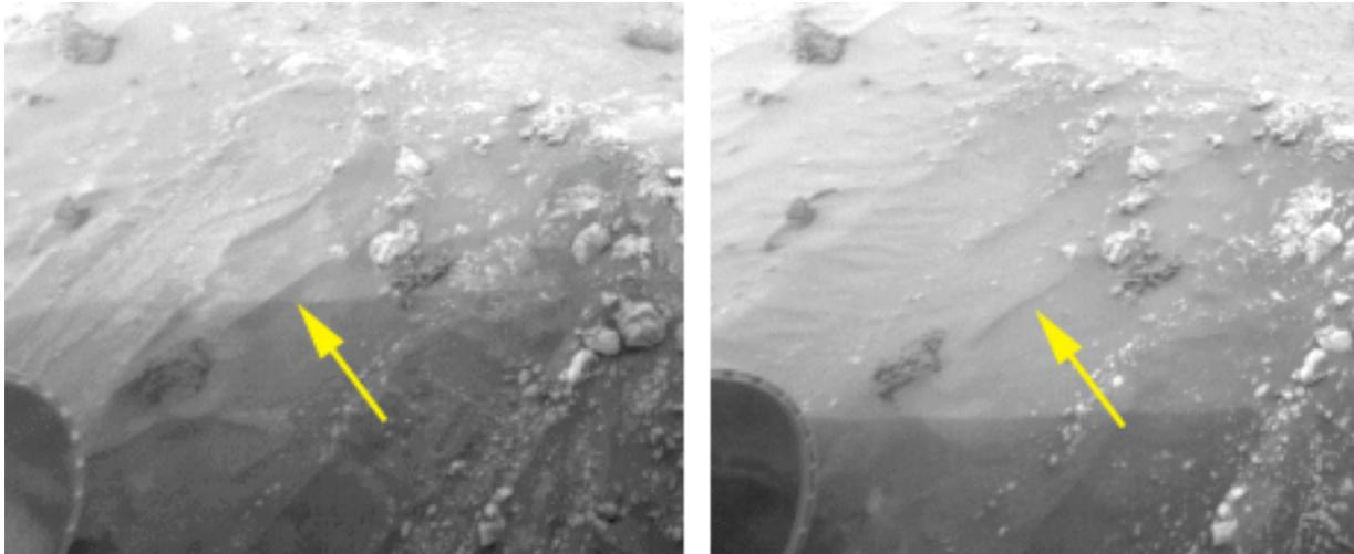
**Figure 1.** Sol 1250 and 1291 front Hazard Avoidance Camera images show ripple crest displacements as large as 2 cm toward the southeast (azimuth 220°). Yellow arrows indicate the ripple crest used primarily for calculations. Rover heading was 50.261° at site 130 position 194.
