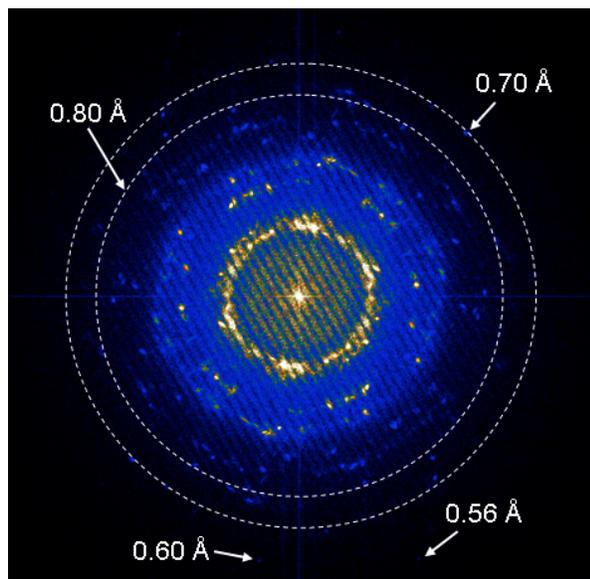
**Figure 1:** FFT of Young's fringe experiment from Au particles on amorphous C. Pattern shows the resolution limit after objective lens correction. The inner dash-line circle corresponds to 0.08nm, the outer circle to 0.07nm. The spots can reach to 0.056nm.
