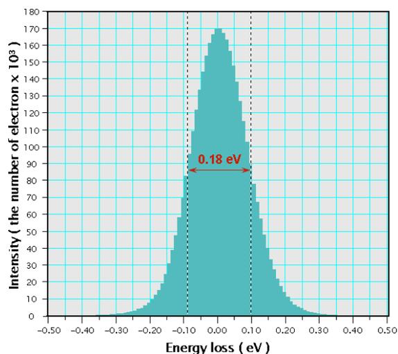
**Figure 3:** 300 keV zero-loss peak with monochromator on and 4200 eV extraction voltage. Energy resolution is 0.18 eV (FWHM) with an acquisition time of 1 second.
