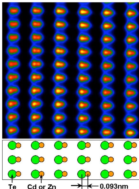
**Figure 2:**  $C_s$ -corrected 300 keV HAADF STEM image of CZT in the [112] orientation showing (Cd,Zn)-Te "dumbbells" (upper) and corresponding schematic of crystal projection (lower). The image demonstrates sub-Ångström resolution.
