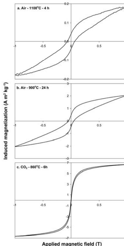
**Figure 1:** Hysteresis cycles of heated nontronite samples obtained using a Princeton Micrometer VSM1. Experimental conditions are indicated on each graph.
