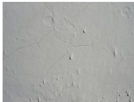
**Figure 2:** Immature cracks; angles are  $\sim 90^{\circ}$ , and cracks do not all connect.
