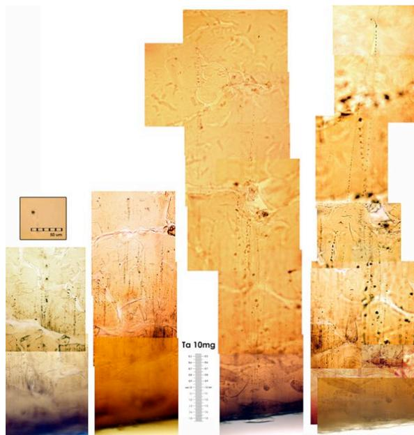
**Figure 2** - Alumina sphere tracks in 10 mg/cm<sup>3</sup> tantala aerogel. The wrinkled appearance of the material is due to minor warping of the aerogel surface.
