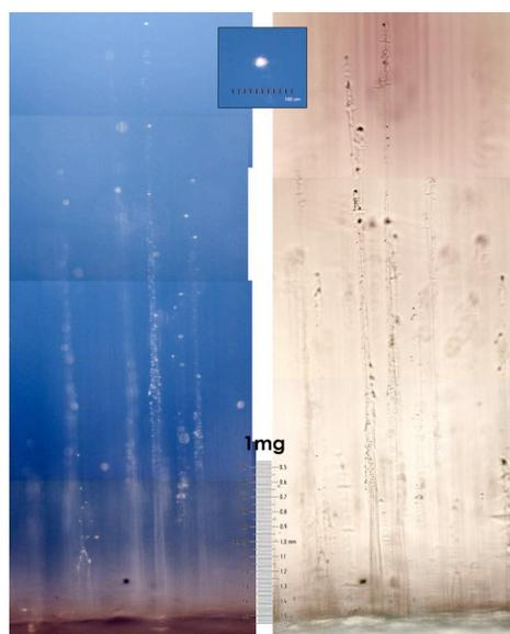
**Figure 1** - Alumina sphere tracks in 1 mg/cm<sup>3</sup> silica aerogel.
